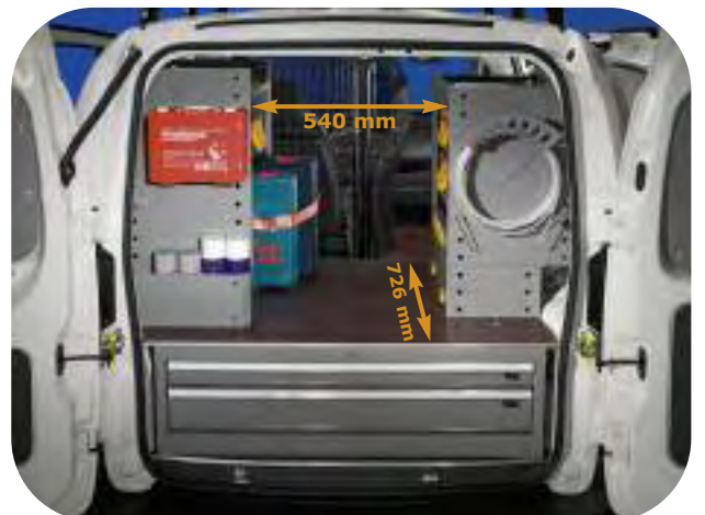
Detail of the double level floor kit with two rear modules
