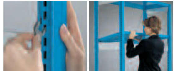
Assembling the strengthening bar and the shelf
