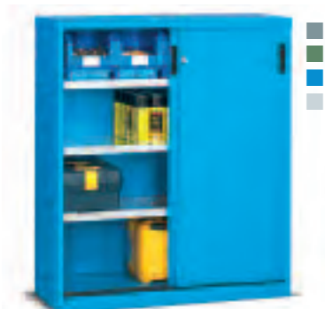
ORD. NO. SHELVES F AB 3200 04 04 3 Cabinet with 3 shelves depth 370 mm load capacity 100 kg Cabinet load capacity: 600 kg Dimensions mm 1023x450x1200 h
