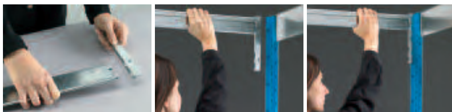
Assembling the strengthening bars
