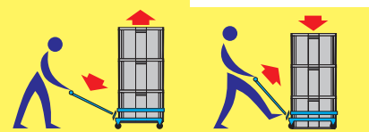
■ how to use the lifting trolley
