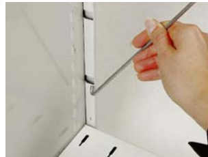
Assembling the cross bracing
